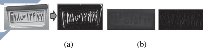
Figure 2: Results of applying the Sobel edge detector on (a) a clean plate and (b) a dirty plate
