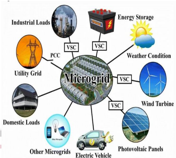
Fig.1 An Illustration of Islanded Microgrid Scheme
