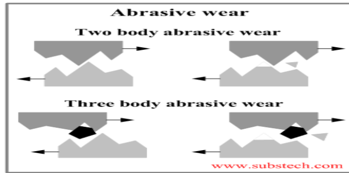
Fig.2 Schematic representations of the abrasion wear mechanism.
