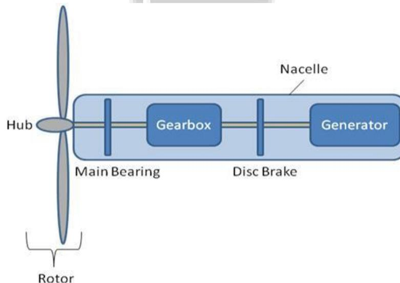
Figure 2 Major Components of a Wind Turbine (Source: Google)
