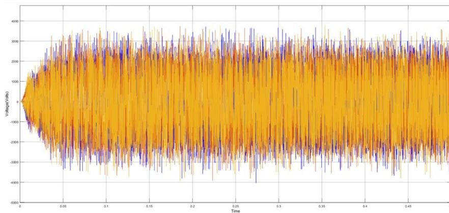
Figure 18 System Voltage Output in the Absence of a Power Controller
