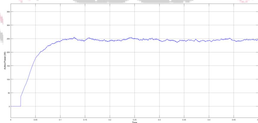
Figure 20 Active Power Output in a System Operated Without a Power Controller
