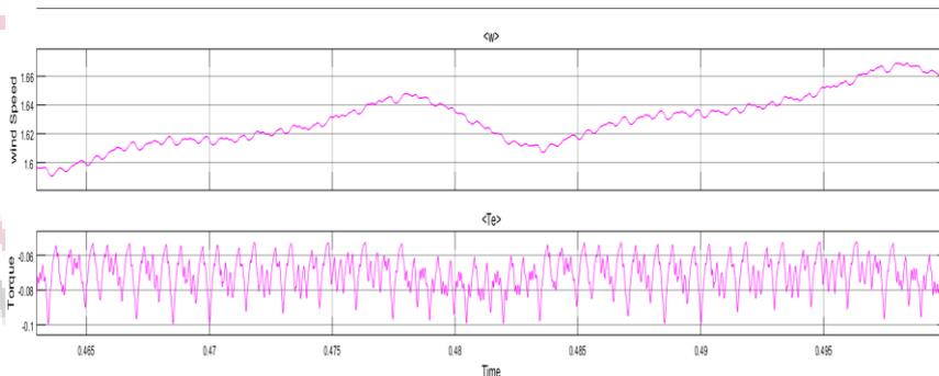
Figure 14 Wind Speed and Corresponding Torque output from the turbine
