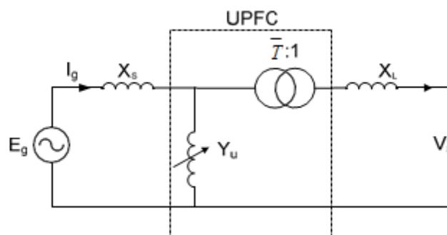
Figure 7 Power system model including UPFC
