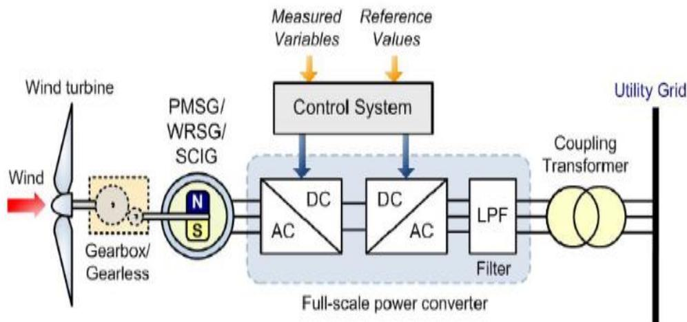
Figure 3 General wind turbine PMSG system with control schemes [5]
