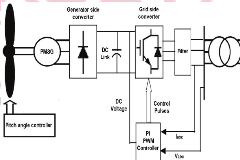
Figure 4 Block diagram of the wind turbine model [7].
