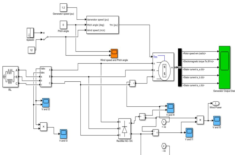
Figure 12 The MATLAB/SIMULINK model of wind energy system
