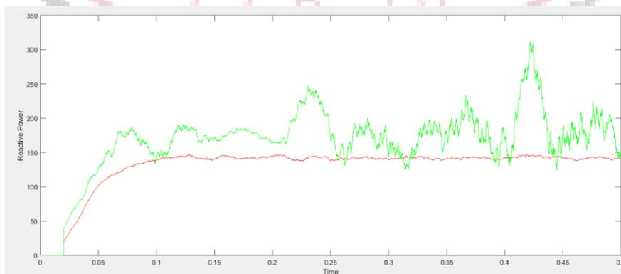
Figure 28 Comparative Assessment of Reactive Power Flow Control
