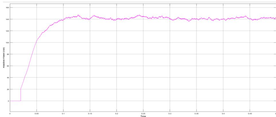
Figure 21 Reactive Power Output in a System Operating Without a Power Controller
