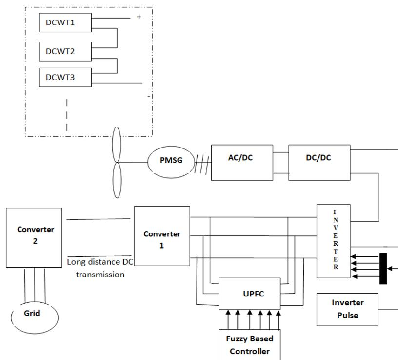
Figure 8 Long Distance DC transmission of Wind turbine system
