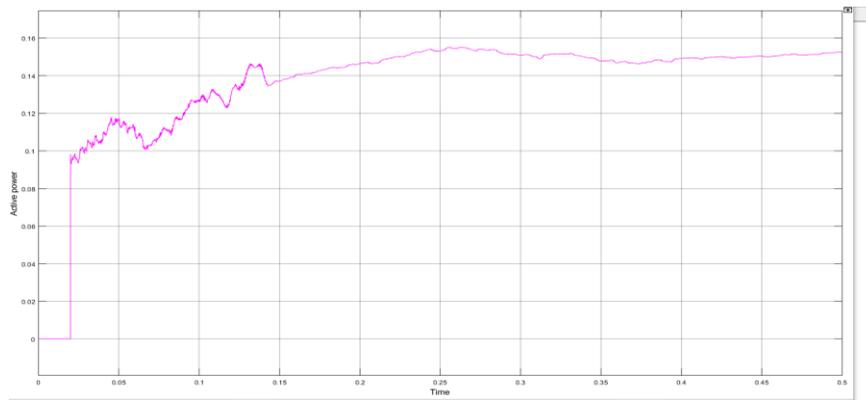
Figure 16 Active power output from DCWT (p.u)
