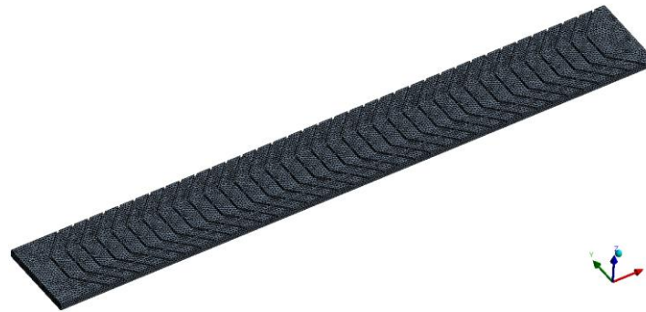
Figure 15 Mesh repair for damaged V-pattern solar air heater the ribs
